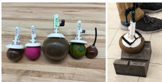
Fig. 2. Membrane in Soft Flexible State vs. Stiffened State
