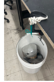
Fig. 8. Shear loading test setup.
